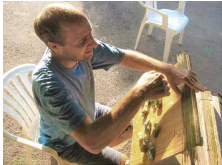
Weaving the screen, Summer 2005. The laid lines are samar reeds; the chain lines are horsetail hair. Garden-hose segments are used as bobbins.
