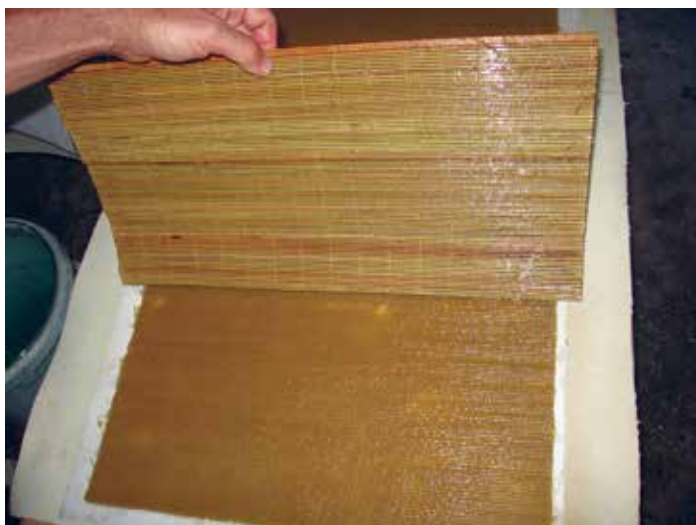
Couching off the paper, Summer 2005. Note the holes in the upper part of the freshly made paper, where the screen was blocked.
