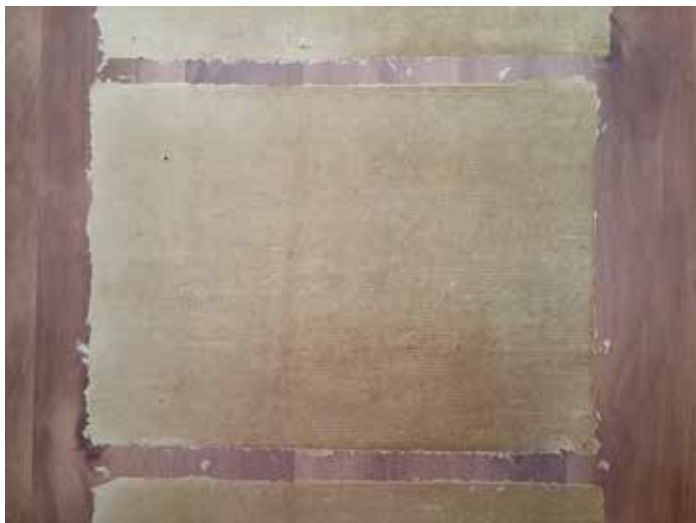
Samar paper drying on Formica boards, Summer 2017. Note the two surfaces of the paper sample—the smooth side faced the board.
