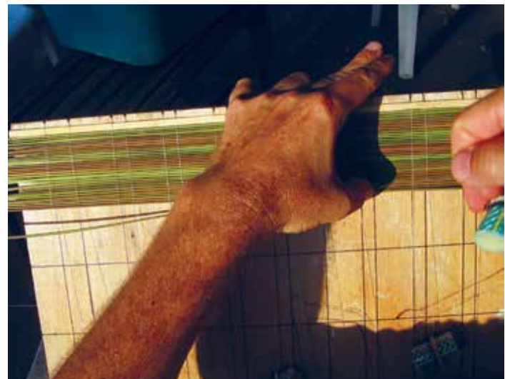
Close-up view of weaving the screen. Note the two different spacings between the chain lines.
